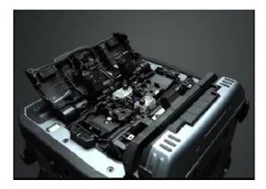
The fiber retention clamps support the automated operations. When the sheath clamps open automatically after splicing, the fiber retention clamps gently hold the spliced fiber to keep it from flying out. The retention clamps release when the fiber is lifted by the operator.
